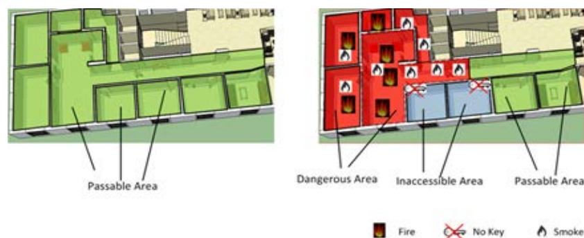
Fig 1: Example of subdivision of space into passable, dangerous and inaccessible area in case of emergency. Before emergency all is 'passable' (left) and during emergency the 'passable' area is shirked to two rooms and a half of corridor (right)
