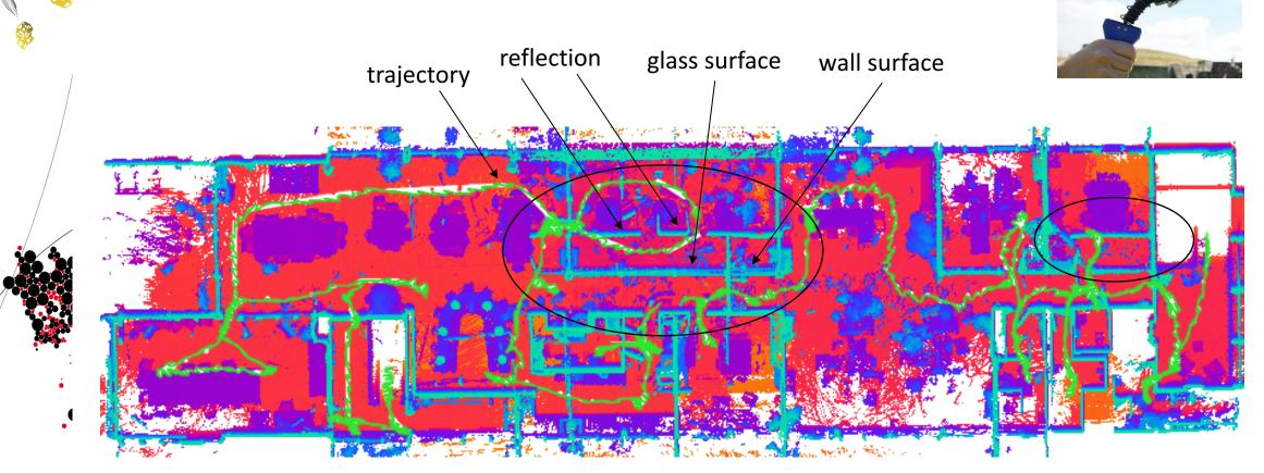
Top view of a room containing reflected surfaces.
